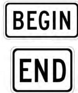
*Figure 7-8 Optional signage for the start and end of bike lanes*
