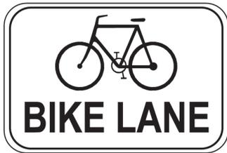
*Figure 7-7 CA MUTCD R81 required signage for Class II bike lane*
