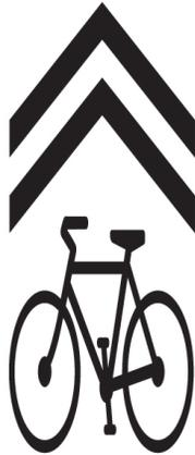
**Figure 7-17** Sharrow pavement marking
