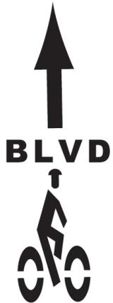
**Figure 7-16** Bicycle Boulevard optional pavement marking
